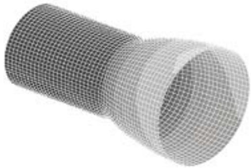
(b) Copper tube under free tube end condition (initial thickness deviation 3.9%)
