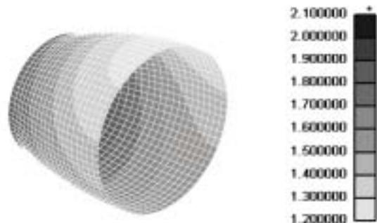
(c) Copper tube under fixed tube end condition (initial thickness deviation 8.5%)
