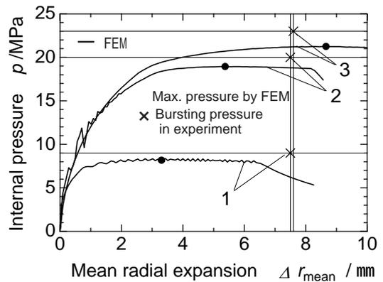
1. Free tube ends with aluminum alloy tube ( $\tau_{ini} = 1.0\%$ )
