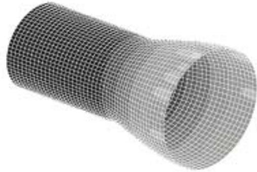
(a) Aluminum alloy tube under free tube end condition (initial thickness deviation 1.0%)
