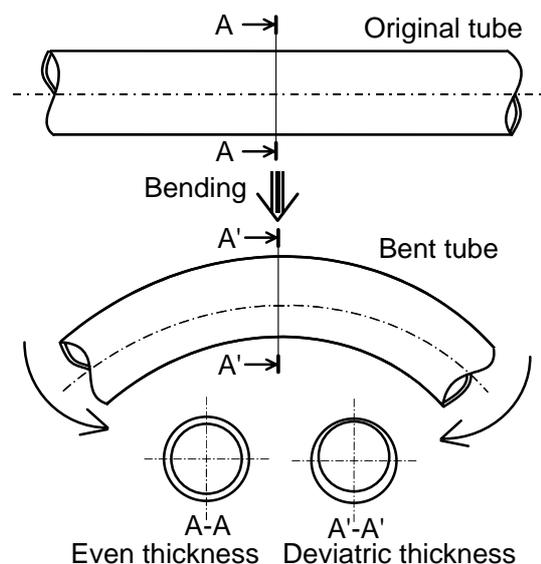
FIG.1 THICKNESS DEVIATION AFTER BENDING.
