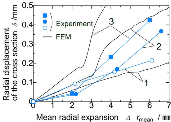
1. Free tube ends with aluminum alloy tube ( $\tau_{ini} = 1.0\%$ )
