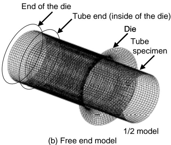
FIG. 5 FEM SIMULATION MODELS FOR THE TUBE WITH INITIAL THICKNESS DEVIATION.
