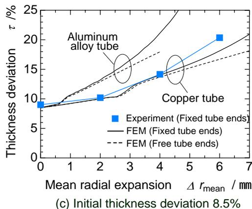
FIG.12 CHANGE OF THICKNESS DEVIATION AT THE CENTER OF THE BULGED TUBE.
